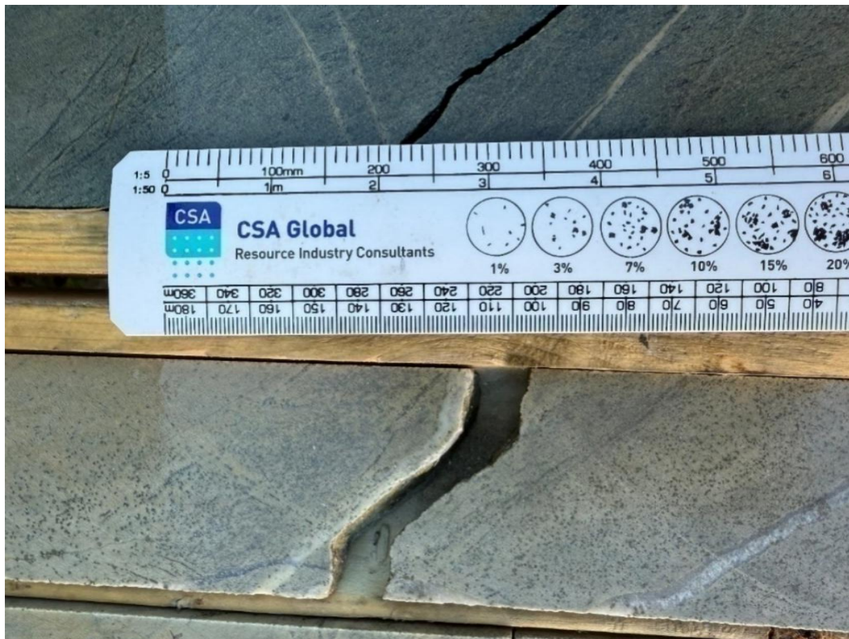
FIGURE 7.2-14 BLEACHED MAFIC VOLCANIC ROCKS WITH DISSEMINATED PYRITE
